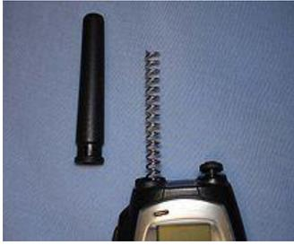
which functions as the needed inductor. The springy wire is flexible, making it less prone to damage than a stiff antenna. The spring antenna is further enclosed in a plastic or rubber-like covering to prevent it from catching on things. Rubber duck antennas are typically 15% to 25% of the length of a standard quarter-wave whip. This antenna is inherently inferior to standard size antennas due to its dramatically shortened length.
