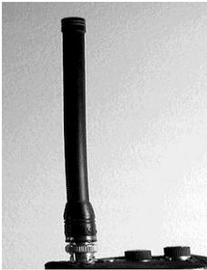
The rubber duck antenna became the antenna of choice for many portable radio devices, including handhelds and portable transceivers, scanners, GPS receivers, and any other device where safety and robustness over long or inflexible whips, takes precedence over antenna capabilities.
